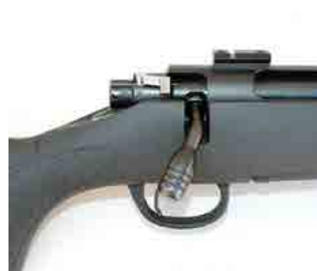
The action of the T/C Compass. The ejection port is well designed for trouble-free case manipulation and the solid bolt with a 60-degree bolt lift and triple locking lugs works very well.
