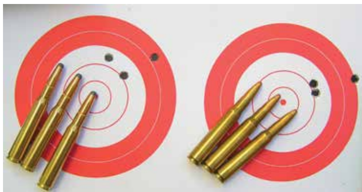
Early 100y groups of 30mm, shot in a cross wind, indicate that they could easily shrink to 25mm on a calmer day with a fully 'run-in' barrel.
