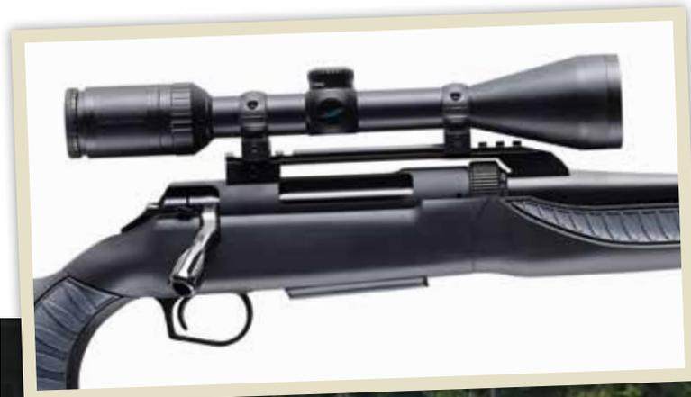
**LEFT:** Not tested but this shows how the TC bridge mount works with the base remaining attached to the barrel by the front of the mount so a scope can be permanently mounted to each barrel.
