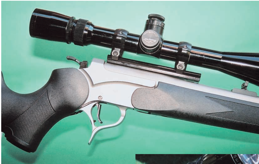
LEFT: The Leupold 6.5-20x Vari-XIII was mounted using a Weaver 410 one-piece base and medium height Millet Steel one-inch rings. Although front of base didn't touch the barrel, it was a rigid system.
