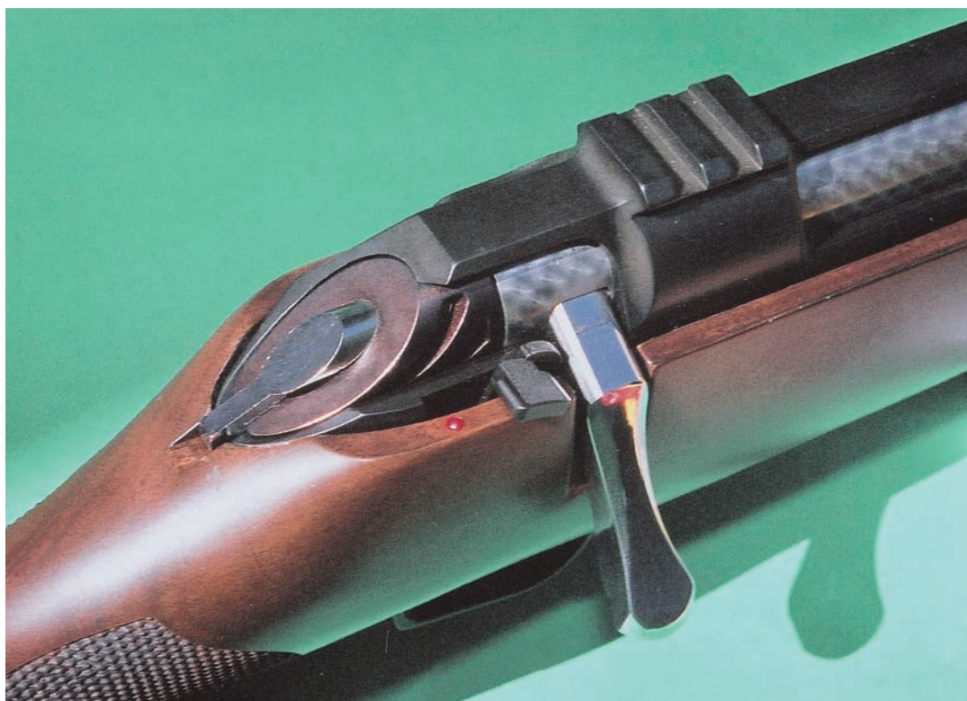
Icon action has integral Weaver-type scope rails with Picatinny cuts and butterknife bolt handle. Note white metal cocking indicator at rear of bolt shroud.
