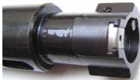
LEFT: The spring loaded sliding extractor operates in a mortise cut into a locking lug.
