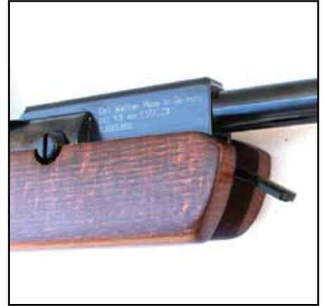
**The chamber block at the breech end of the barrel mates up with the end of the piston chamber. The rifle's calibre and serial number are located on this block. The larger screw is the pivot point, which the barrel hinges on. The wedge lock release lever is clearly shown on the front of the stock.**
