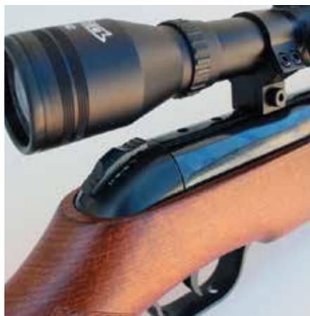
**The safety tab on the receiver tang of the Walther Century. The safety was automatic, being engaged each time the rifle was cocked. Sliding the tab forward to 'F' meant the rifle was ready to fire.**
