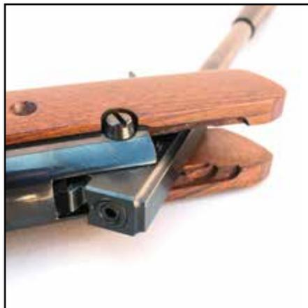
**The loading port for the .177-calibre pellets. The O-ring is of high-quality rubber and positively seals the chamber against the piston assembly. It ensures all the compressed air in the piston travels up through the barrel propelling the pellet and is not lost elsewhere along the line.**
