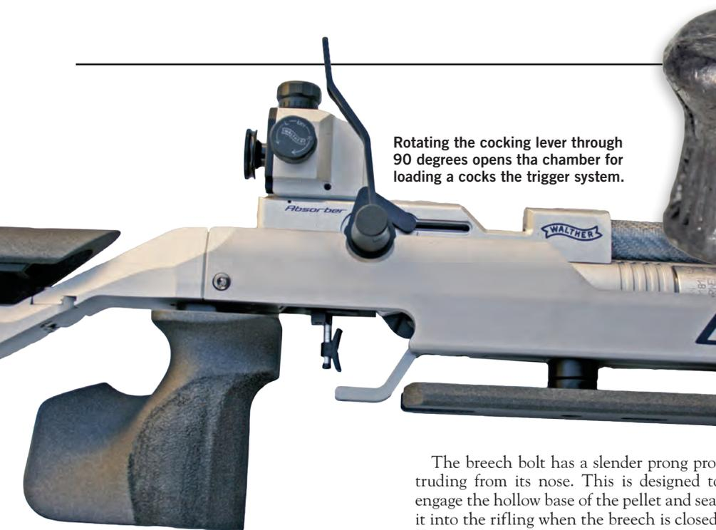
Rotating the cocking lever through 90 degrees opens the chamber for loading a cock the trigger system.
