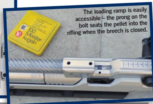
The loading ramp is easily accessible – the prong on the bolt seats the pellet into the rifling when the breech is closed.
