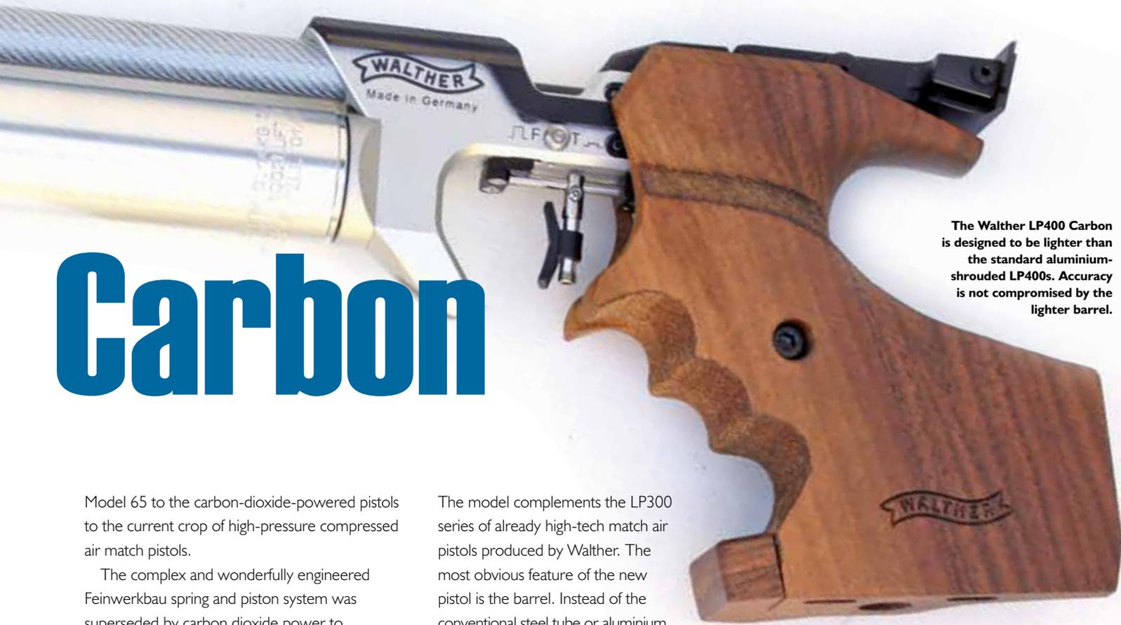
The Walther LP400 Carbon is designed to be lighter than the standard aluminium-shrouded LP400s. Accuracy is not compromised by the lighter barrel.
