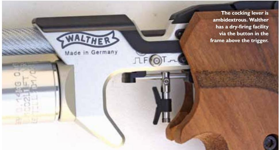
The cocking lever is ambidextrous. Walther has a dry-firing facility via the button in the frame above the trigger.
