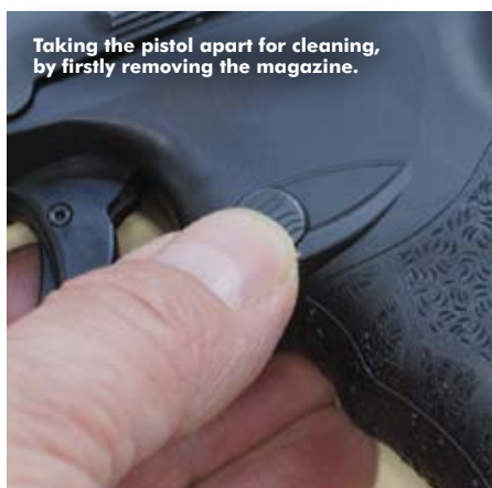
After dry-firing, the take-down latch is lowered.
