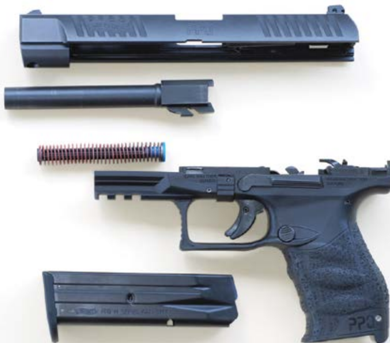
The pistol dismantled into its five main sub-assemblies.
