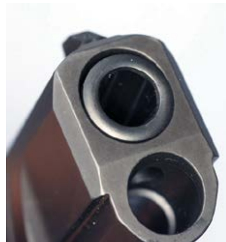
The muzzle up close, showing the oval hole in the slide that enables the barrel to tilt during unlocking.
