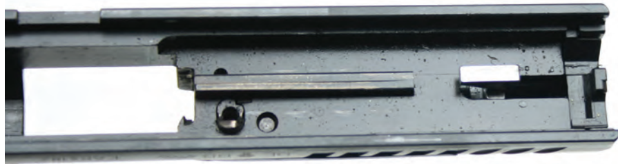
The striker firing system on the PPQ results in a very clean and simple slide arrangement.
