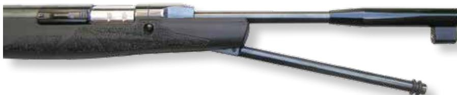
**BELOW:** Two of the piston safety stops are visible on the closed compression tube in front of the safety release toggle.
