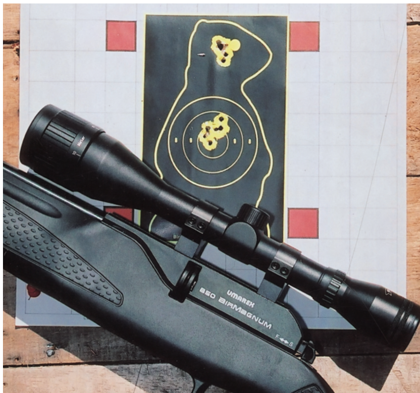
The accuracy of the Umarex 850 Airmagnum can be judged by these two 8-shot groups shot at 25 metres with Umarex pellets.
