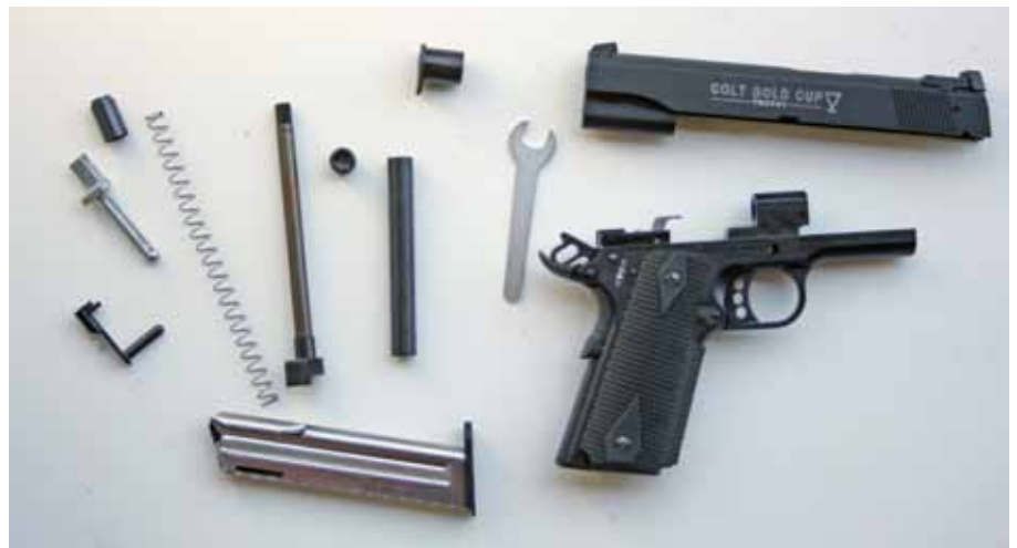
ABOVE: The Gold Cup stripped. The barrel is held in place with a shroud and barrel nut and can be completely removed from its fixed position in the frame.
