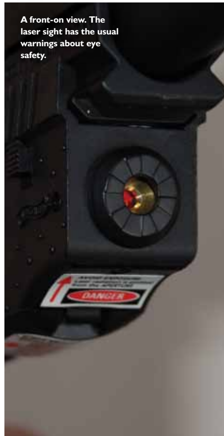
The laser sight up close. The on/off switch is within easy reach of the trigger finger. Windage and elevation is adjusted via a supplied hexagon key.
