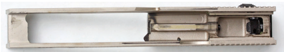
The satin-nickel-plated slide appears to be a precision investment casting.
