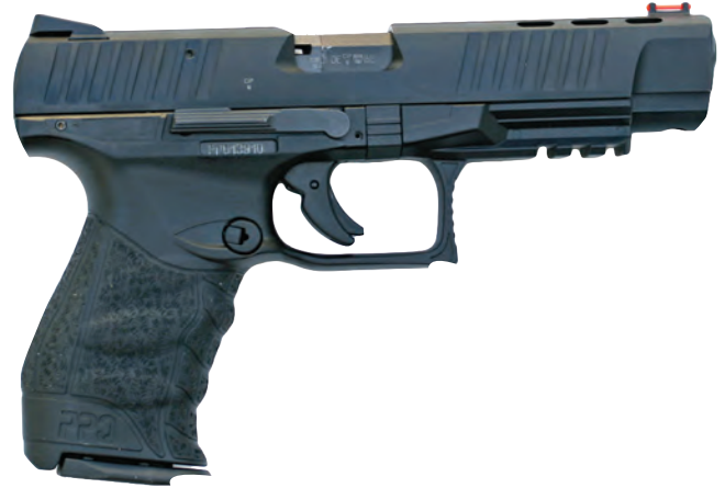
FROM LEFT TO RIGHT: The PPQ .22 with temporary trigger stop (double sided foam tape) fitted. The PPQ .22 has no conventional safety. The blade in the trigger does that job, preventing the pistol from operating until it is fully depressed.
