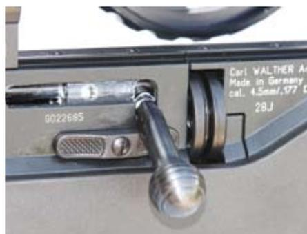
**The eight-shot magazine is now in place and the bolt is closed. One merely has to release the safety catch and the gun is ready to fire.**
