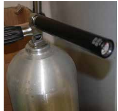
Charging the cylinder from a scuba tank - maximum pressure is 200 Bar.
