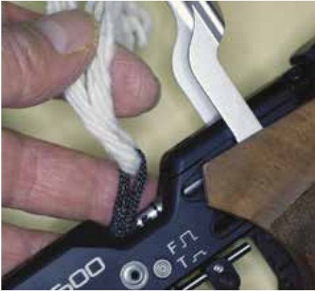
Pulling cleaning strings through the bore.
