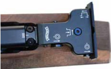
Top view of the rear sight, adjustable for windage, elevation and width.
